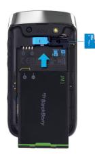
To remove the media card, press the media card in and then pull it out.
